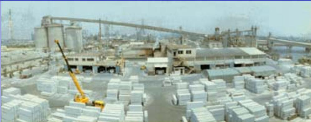
The weight and texture of concrete block depend largely on the type of aggregate used in its manufacture. Block made with sand and gravel and crushed stone weighs from 18-22 kg. These blocks are strong and durable, with a low absorption rate, blocks made with light weight aggregate weigh 11-16 kg. Light weight blocks are produced as non-bearing units, for use as backup walls or load-bearing units, for use as the finished surface of both interior and exterior walls.
